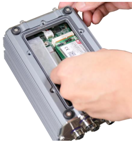
Insert at 45 degree angle
