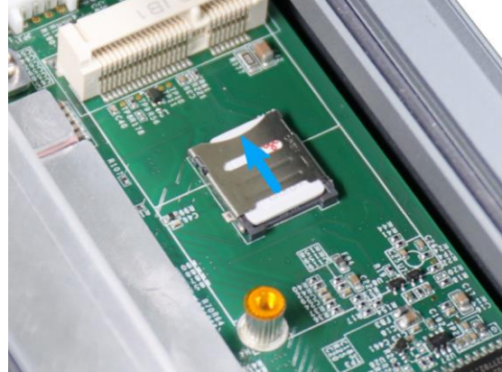
Slide to secure SIM and bracket
